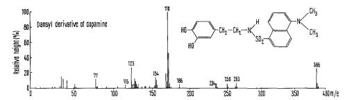
Mass spectrum of the dansyl derivative of dopamine, isolated from the carotid body of the horse (Hitachi-Perkin Elmer RMU-6D mass spectrometer, direct inlet, 70 eV, 365 °C).
